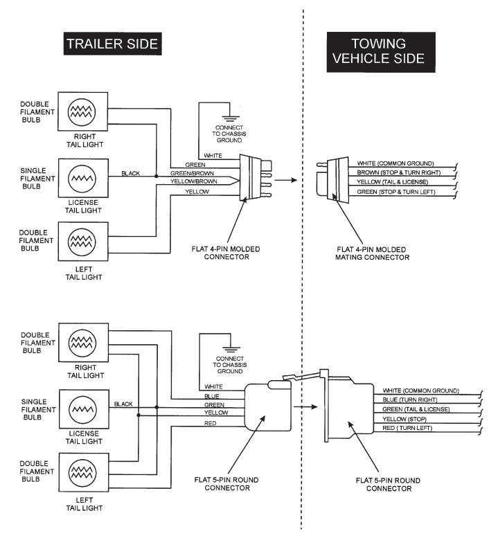
Figure 47. Trailer/Towing Vehicle Wiring Diagram
